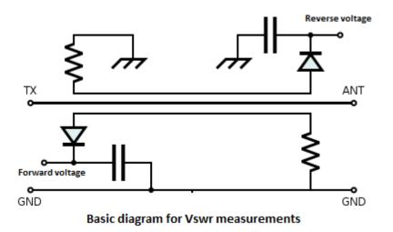
The subject of impedance measurement of antenna's, i.e. aerial's, is the Voltage standing wave ratio measurement. The load impedance "ZL" is the first to find, from this the fraction value or the "row" value is found. This will determine if the load impedance is greater or lower than the object impedance "Zo", the row value then negative in magnitude if the "ZL" value is less than the "Zo" design value, and positive magnitude if "ZL" is greater than "Zo".
