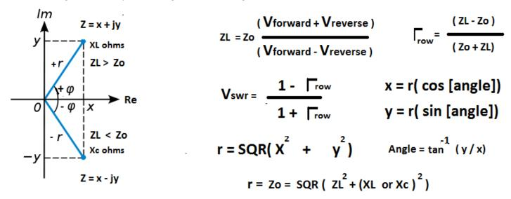
Should the row value be positive, then the resultant vector "+r" angle, would indicate an inductive loading, or an antenna with too a high impedance. Example, if "ZL" = 52ohms, then the vector angle is +15 degrees, while if "ZL" is 48 ohms, then the angle is -16 degrees, indicating a too lower impedance and a capacitive loading. These vector angles are relative to the 50ohms design impedance, thus the magnitude value of a polar rectangular equation.
